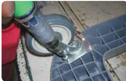
Using the T40 Torx driver, unscrew all four bolts.
