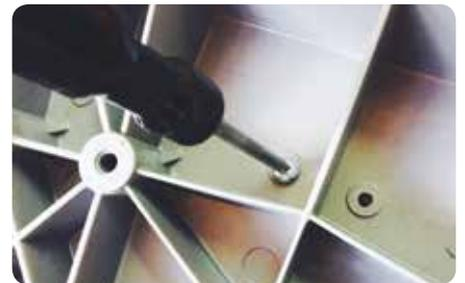
Turn trolley upside down and screw in all 8 self-tapping screws.
