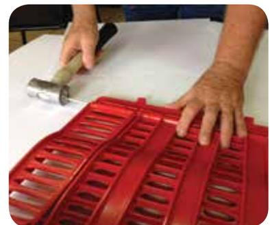
Insert rod into hinges and tap in with mallet.
