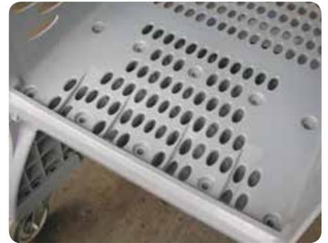
There are 10 plastic rivets that need to be inserted to attach these two components.
