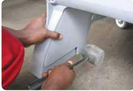
Press down so that sides are flush. Using a mallet, gently knock into place until you hear a click.
