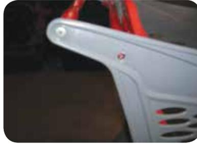
Drill out existing rivets with a 6.5mm drill bit. Remove the old backgate assembly.
