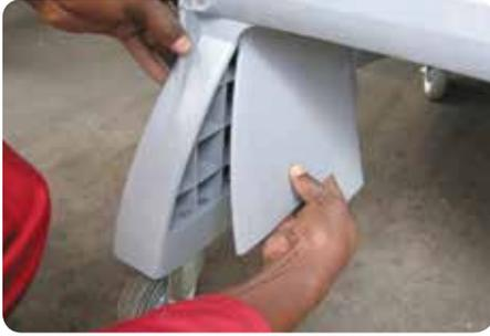
Ensure the side cover is placed correctly, starting from the top.
